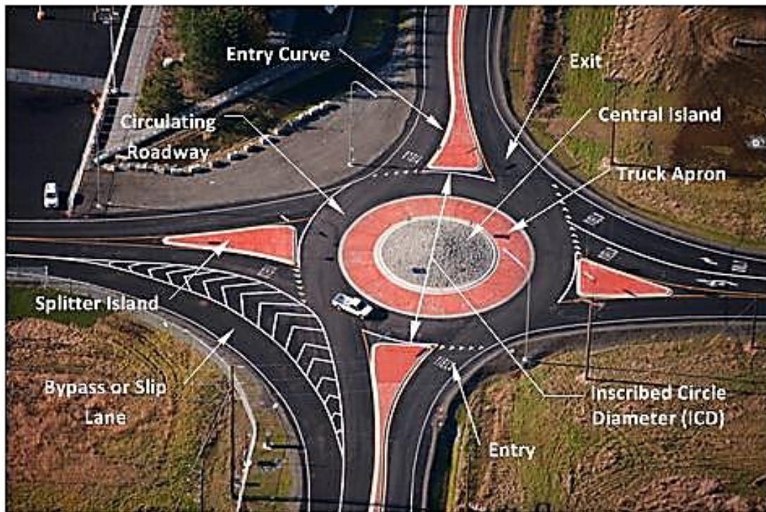
Roundabout design elements
